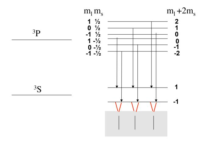
Six transitions give three lines due to degeneracy as splitting  $\propto (m_l + 2m_s)$
